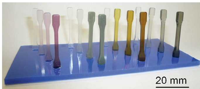
Figure 4: Injection-molded prototypes made of laser-generated polyurethane nanocomposite with different nanoparticles (from left: gold, zinc oxide, silver, copper)
