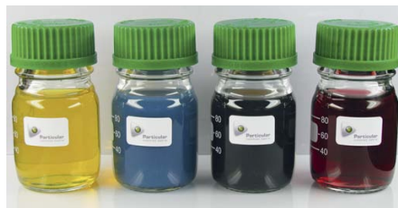
Figure 6: Colloidal diversity of laser-fabricated nanoparticles (from left): nanoparticles made of silver, titanium, platinum and gold in acetone
